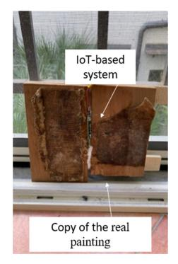
Figure 4. Prototype under test, copy of *The Deposition*.
