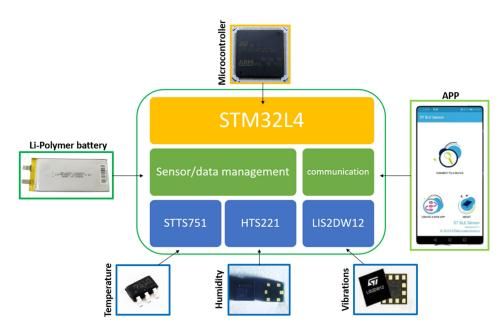
Figure 2. Schematic diagram of the IoT-based system for microclimate monitoring.
