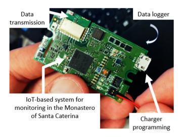
Figure 3. Board used for the monitoring of the painting.
