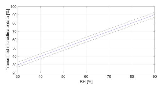
**Figure 7.** Characterization in terms of relative humidity at 20 °C.
