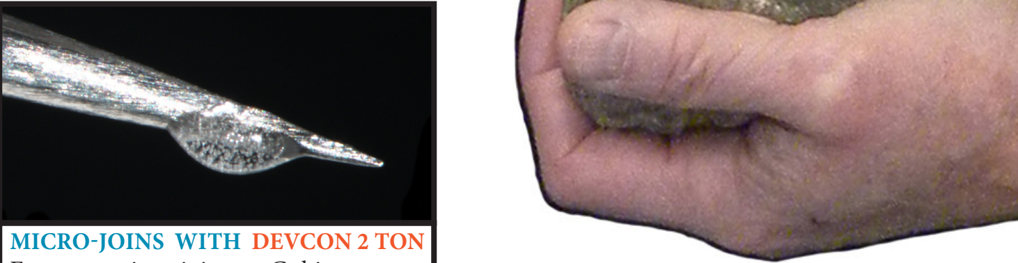
MICRO-JOINS WITH DEVCON 2TON For most micro-joins on Gobi specimens (e.g. below), slow set-time is a priority for manipulating and adjusting the join before the adhesive sets. Devcon 2 Ton is not as removable as any of the solution adhesives (e.g. Paraloid B-72), but it is easy to apply in tiny drops (above) that set slowly regardless of amount. Solution adhesives dry up very quickly in tiny drops & are more difficult to manipulate for micro-joins.
