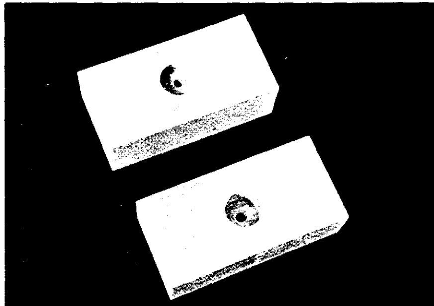
Figure 11. Empty "block" samples. Holes are 1" wide and either \frac{3}{4} " or \frac{1}{2} " deep. (Photo: Author)
